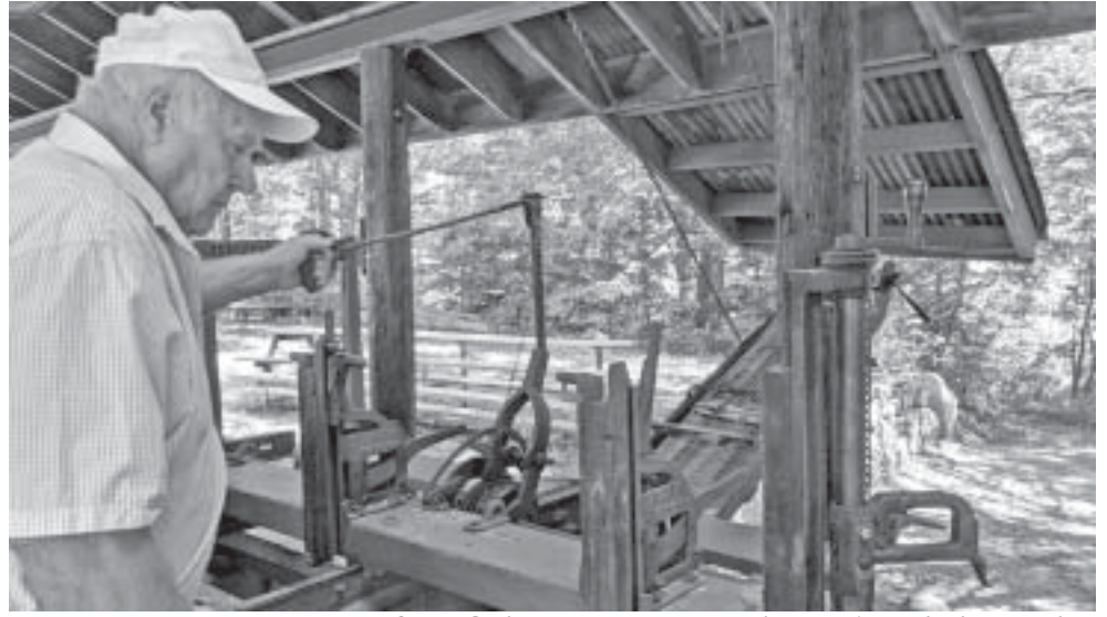
Ned Tewksbury, member of the Quinebaug Valley Engineers Association, which owns and runs the Zagray Farm Museum in Colchester and Hebron, cranks a Double Acting Dog on an 1878 sawmill. The device was invented by Stanley Zagray, the eldest of three brothers who owned and operated the property when it was an active farm.
